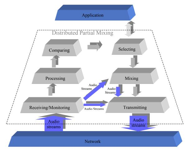
Figure 3.4 Functional model of Distributed Partial Mixing
