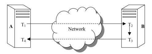
Figure 4.3 Calculating network distance
