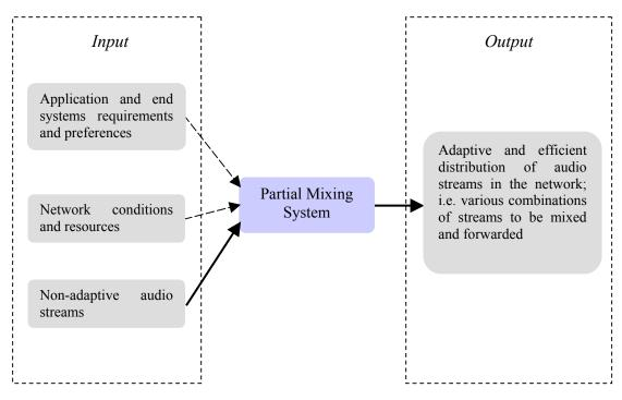
Figure 3.2 Input and output of a partial mixing system
