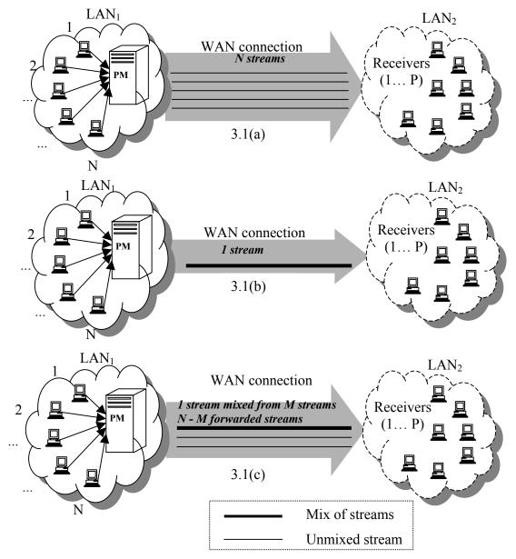
Figure 3.1 Small-scale partial mixing example
