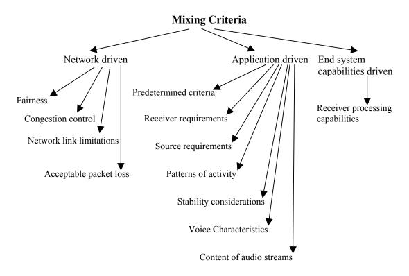
Figure 3.5 Scheme of various types of mixing criteria
