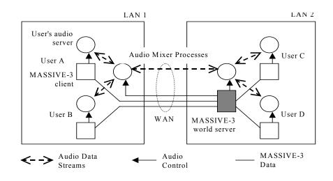
Figure 4.4 An example of distributed partial mixing in MASSIVE-3
