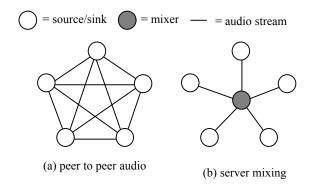
Figure 2.1 Logical model of peer-to-peer vs. server based approaches for distribution of audio streams
