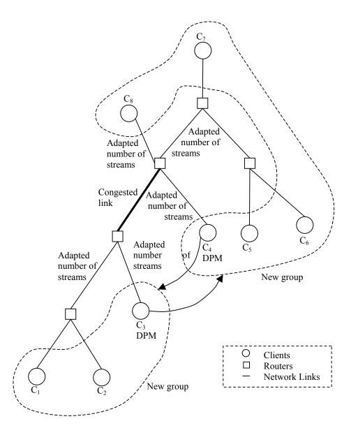
Figure 5.6 Partitioning the original multicast group into multicast islands when the problematic link is congested in both directions
