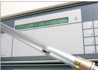
Fig. 3-5 Burst pressure test
