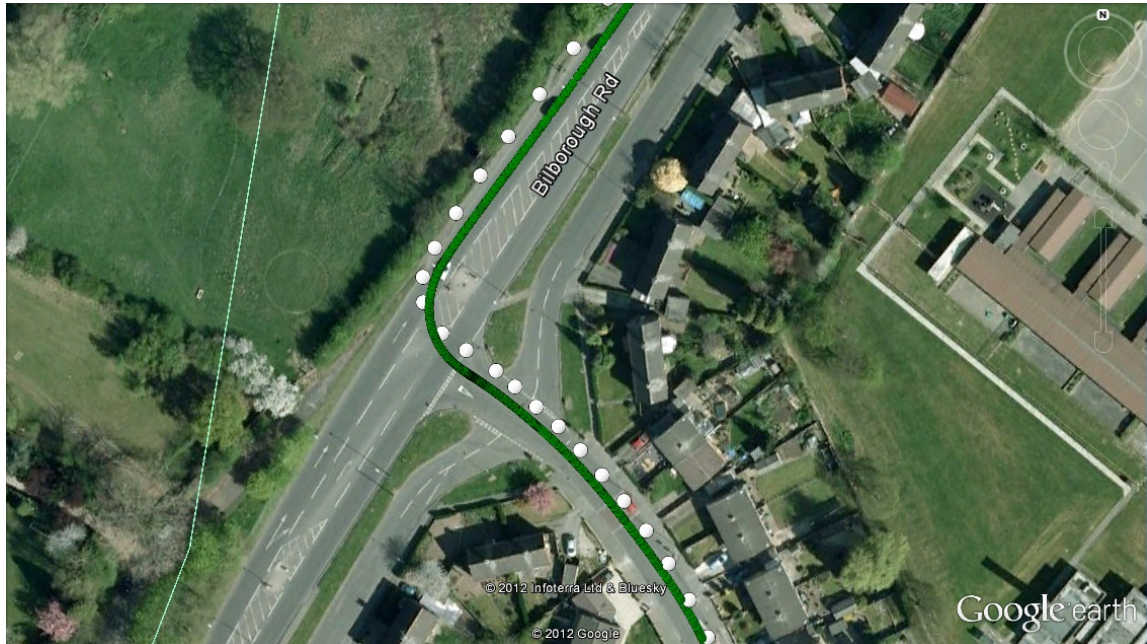
Figure 1.11 – The positioning performance of a Sat Nav device (white) compared to a high precision GNSS receiver (green).
