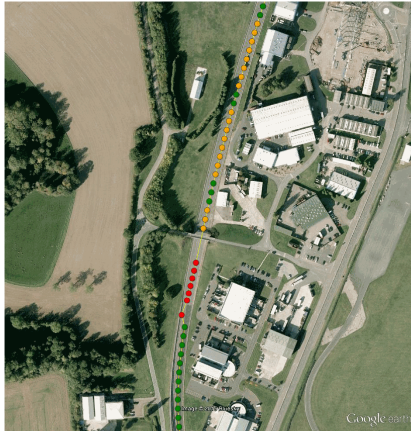
Figure 5.3 – N-RTK GNSS signal outage at MIRA proving ground - No.2 circuit.
