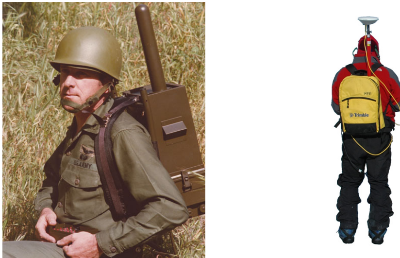
Figure 4.4 – GPS receivers then and now. Left: An early GPS receiver Manpack. Right: The latest Trimble GNSS backpack.
