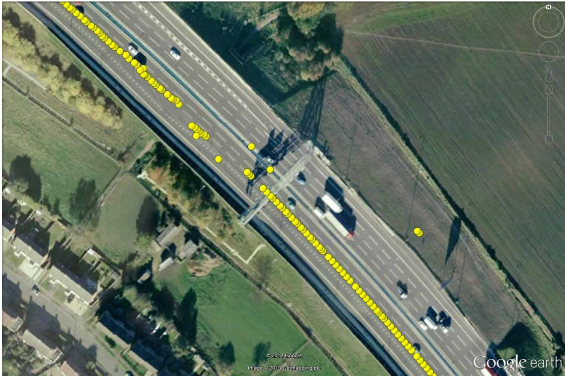
Figure 5.5 – The typical effect of overhead obstructions on GNSS positioning of a road vehicle.
