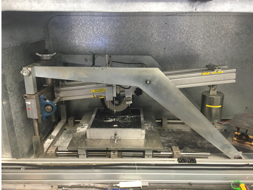
Figure 6.2: Wheel Tracking Machine
