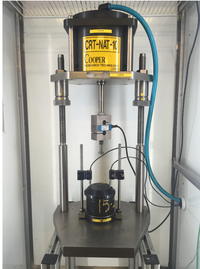
Figure 6.3: RLAT Testing Machine
