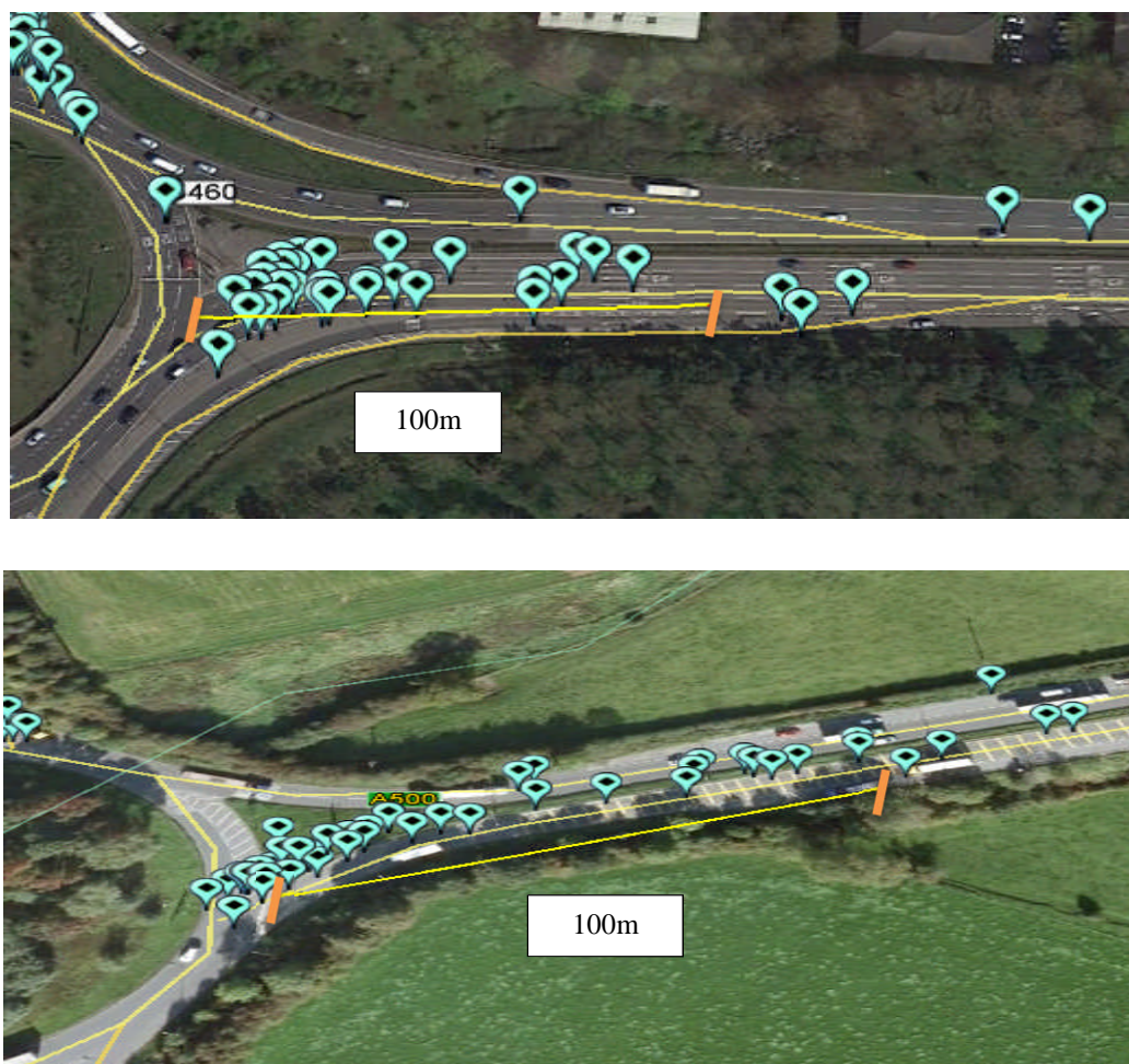
Figure 3-10 Harsh Braking Locations and 100m Distance From Entry Line, East of J21 on the M1 and East of J16 on the M6, Respectively
