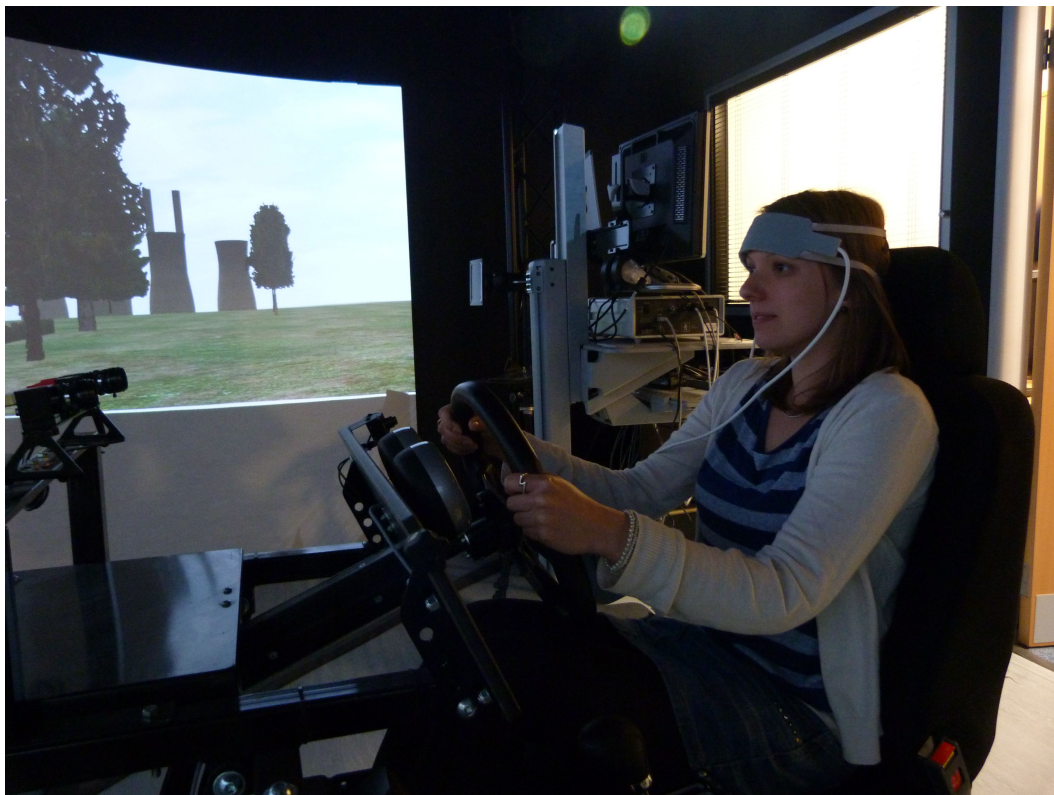
Figure 6.2. NITES 2 driving rig and a participant with the fNIR sensor on their forehead.
