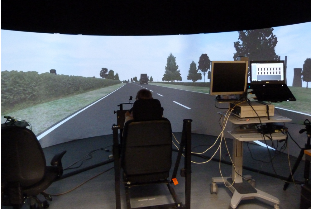
Figure 6.1. View of the NITES 2 driving simulator with the driving rig (centre) and fNIR device (right).
