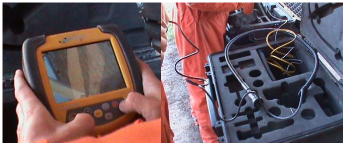
Figure 45 - SnakeEye monitor (left) and goose neck extension (right)
