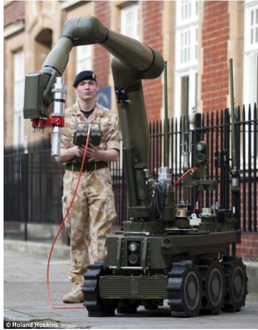
Figure 1 - CUTLASS Bomb disposal robot used by the British Army ("CUTLASS EOD robot [Image]," 2012)
