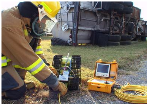
Figure 8 - R2i2 Delta Extreme from RECCE robotics ("R2i2 Extreme [Image]," 2015)
