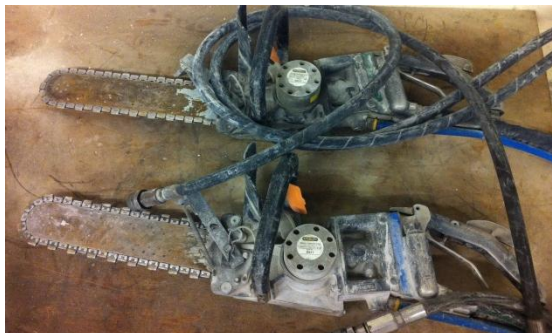
Figure 53 - Hydraulic concrete chain saw
