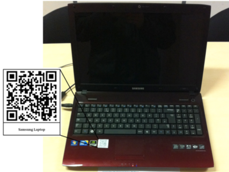
Figure 3.4: Laptop client device with MultiNet QR Code encoded credentials.
