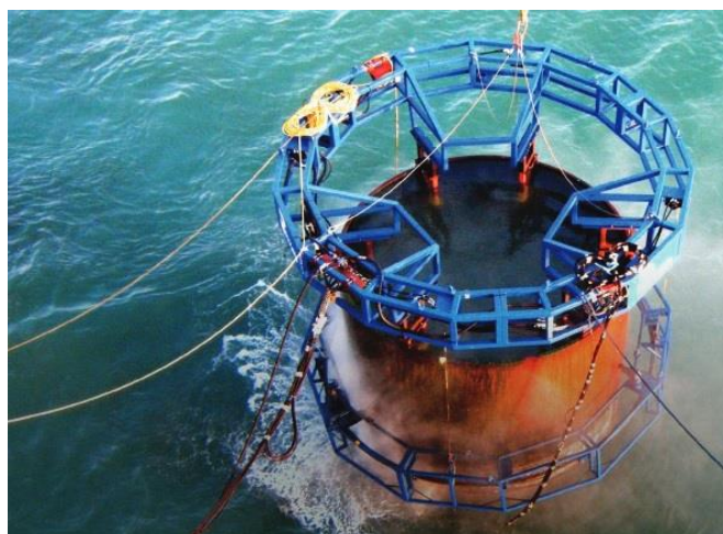
Figure A-10, Proserv marine growth removal (MGR) tool (Proserv, 2014)
