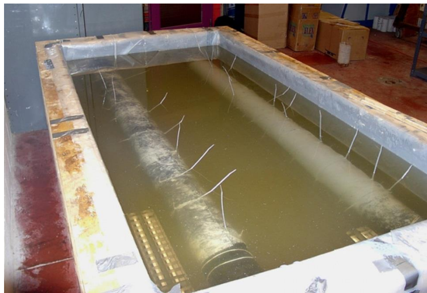
Figure 2-20, FRPC-wrapped specimens cured under saltwater conditions (Seica & Packer, 2007)
