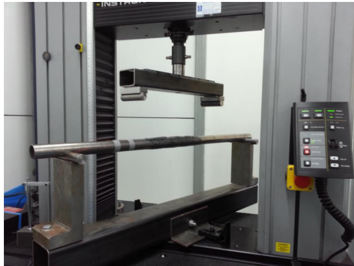
Figure 5-5, Four-point bending setup with the aid of an Instron load frame
