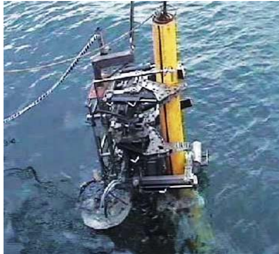
Figure 2-7, Prototype of the unmanned underwater robotic crawler (Chatzakos, et al., 2010)
