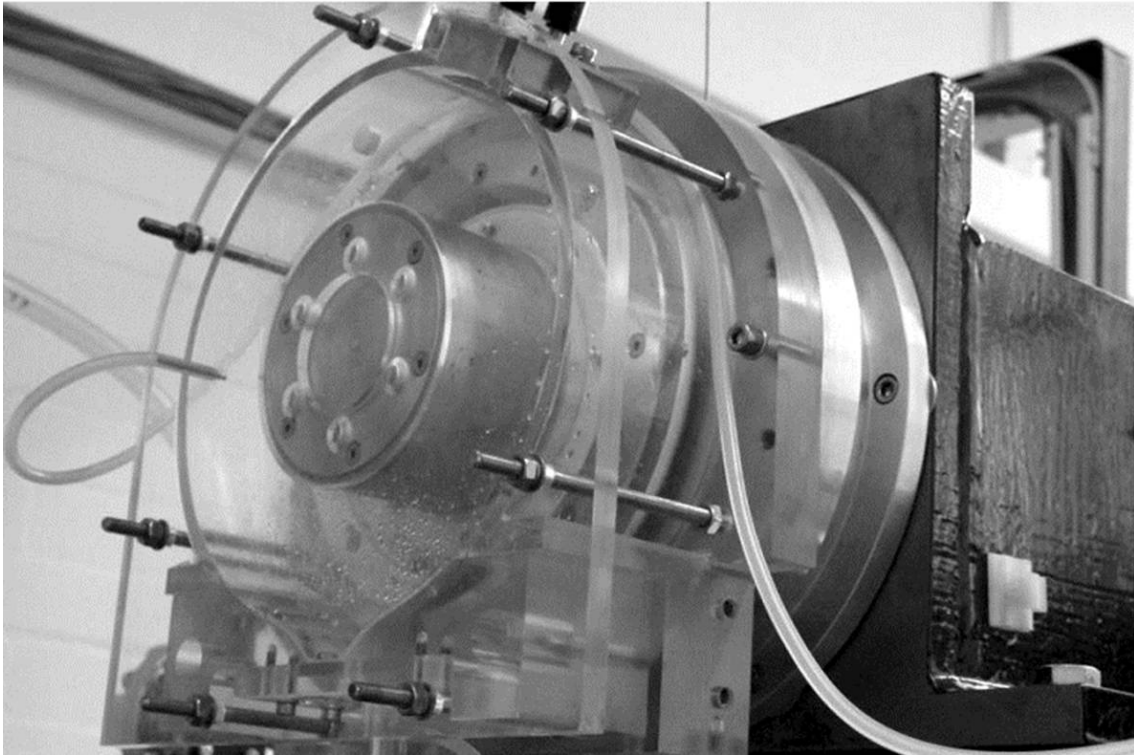
Figure 6.2: Bearing chamber with Perspex see-through wall
