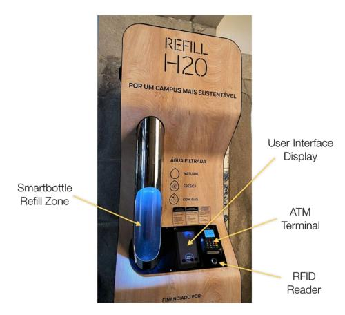
Figure 6. Refill Station with identification of main elements.
