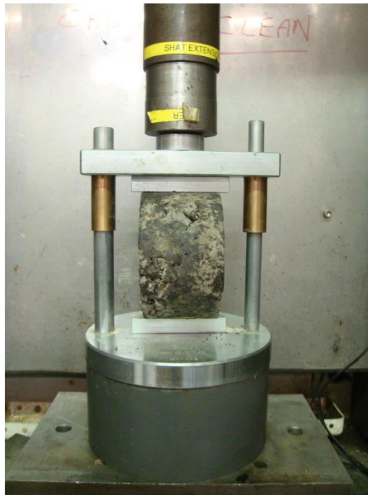
Figure 6.3 ITS test equipment
