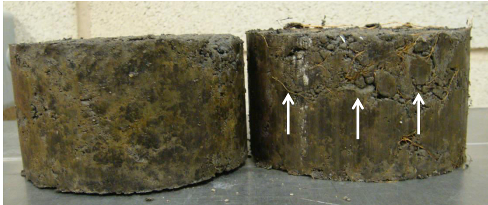
Figure 9.2 Compacted foam mix with and without coir fibres
