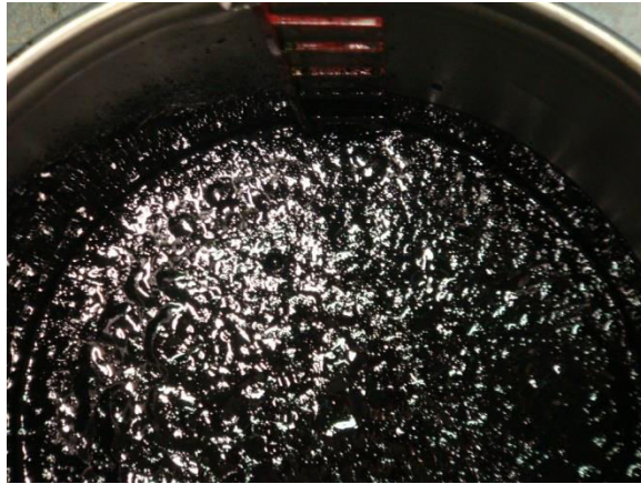
Figure 7.2 A red dip stick with prongs measuring the maximum height of foamed bitumen
