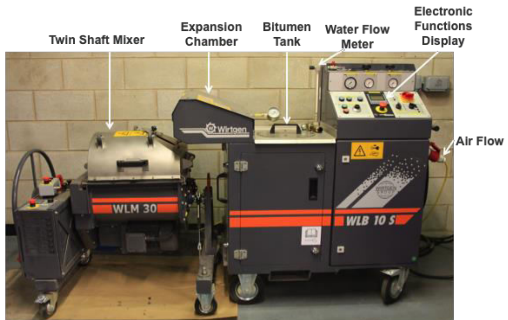
Figure 7.5 Foamed Bitumen Plant, WLB 10s, coupled with a Twin Shaft Mixer
