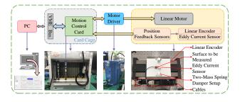
Fig. 6: Block diagram of the experimental setup.
