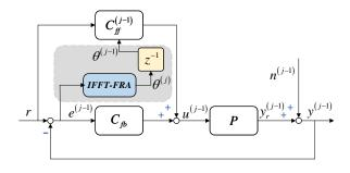
Fig. 1: Two-degrees-of-freedom control configuration with IFFT-FRA tuning algorithm. The symbol z denotes the forward shift operator with respect to iteration and the superscript j denotes the iteration index.
