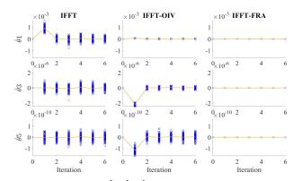
Fig. 4: Parameter  $[\hat{\theta}_1, \hat{\theta}_3, \hat{\theta}_5]$  as a function of iteration for M = 100 realizations for IFFT (left), IFFT-OIV (middle) and IFFT-FRA (right). Their ideal results are thought to infinitely approximate to **0**.
