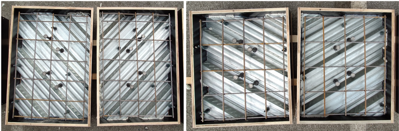
Figure 4.9: Specimens D45 and D60 before concrete casting.
