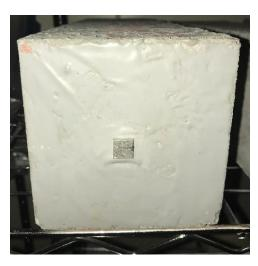
Photo 3.4 The gauge plug in the specimen
