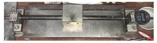
Photo 3.5 Drying shrinkage test equipment
