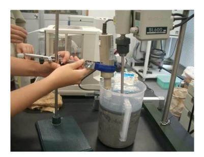
Figure 4.2. Microbubble generator.
