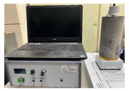
Picture 6.2. Test device for  $E_d$ .
