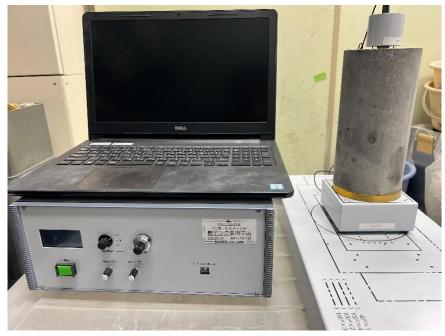
Photo 3.6 Dynamic elastic modulus test machine.
