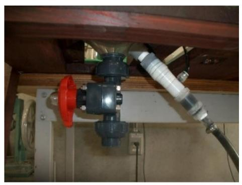
Figure 3.3. Microbubble circulation device.
