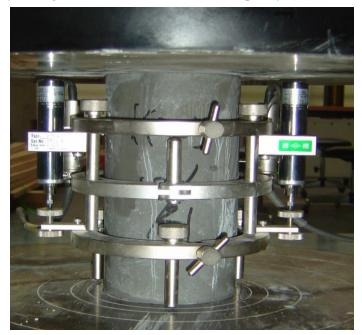
Picture 6.1. Test setups for  $E_c$ .
