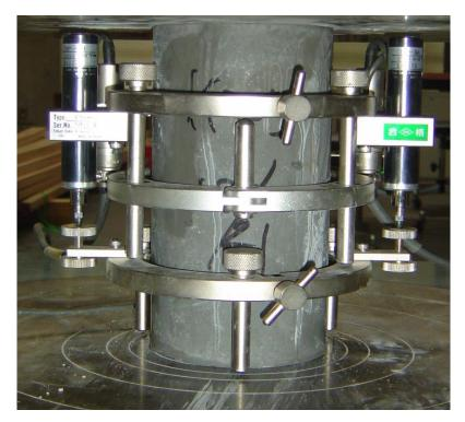
Fig 3.6 Static Modulus Apparatus Consisting of Compressometer Gage (Dial Gage) and Extensometer Gage (Digital Gage)
