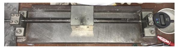
Photo 7.2 Drying shrinkage test equipment
