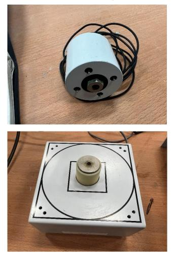
Photo 3.7 Resonance vibration machine
