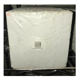
Photo 7.1 The gauge plug in the specimen
