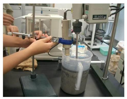
Figure 3.2. Microbubble generator.
