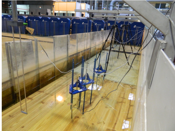
Figure 4.12: Wave gauges setting for the subset B25 experiments.
