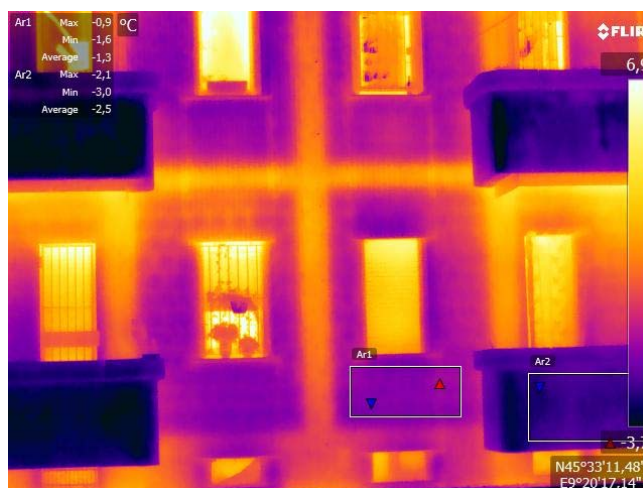
Figure 6. Graphic definition of the areas of the wall to evaluate the average temperatures to be considered.
