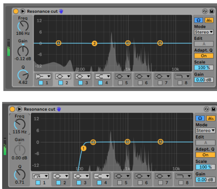
Figure 4.5: Before and after images when rolling off low frequencies with a hi-pass filter taken from the mix, “French Connection.”
