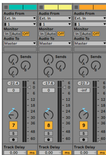
Figure 4.15: Three separate audio tracks with the differing stereo panning decisions represented by the light blue markings (read from left to right, approximately 60 percent to the left; 25 percent to the left; and 25 percent to the right).
