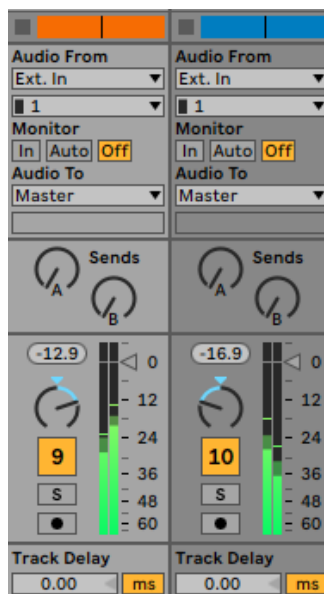
Figure 4.14: The highlighted light blue areas within the clock-like symbols are the panning settings within Ableton's tracks. These variables allow users to pan audio tracks from left to right.
