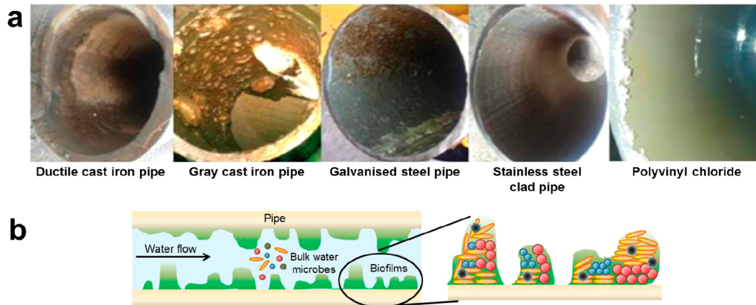
Figure 6: (a) Images showing biofilm growth on different pipe materials. Reprinted with permission from [94]. Copyright 2015, Springer Nature. (b) Representation of a biofilm life cycle, including their possible resuspension. Reprinted with permission from [2]. Copyright 2016, American Chemical Society.
