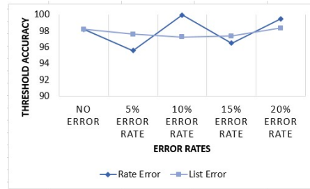
Fig. 9. Accuracy of leakage detection in HPN
