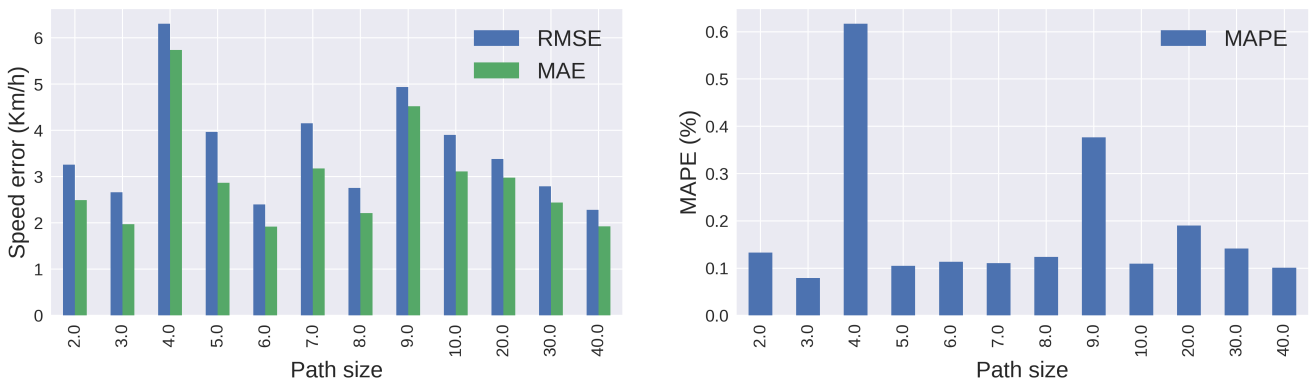
Figure 9: Evolution of the error (RMSE, MAE, MAPE) of compositional predictions depending on the number of inter-stations. Each sub-line is extracted from consecutive inter-stations of line 858.
