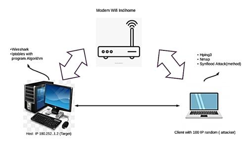
Figure 9. Attack Simulation Schematic
