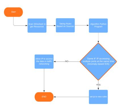
Figure 4. Flowchart Algorithm
