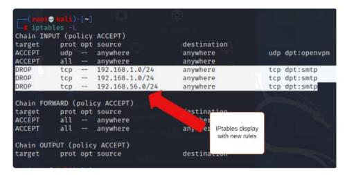
Figure 8. Display of new IP tables rules
