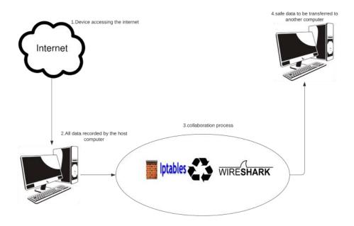
Figure 2. Wireshark-Iptables Collaboration System Design
