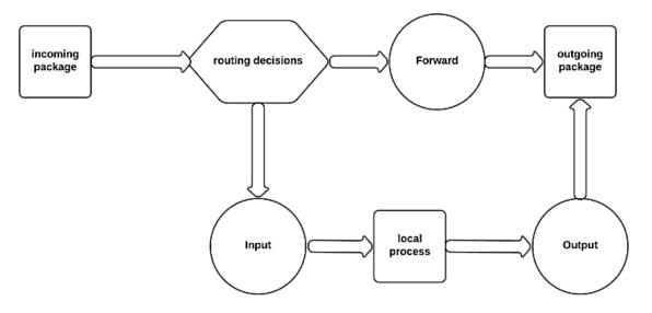
Figure 1. Filtering system on Iptables
