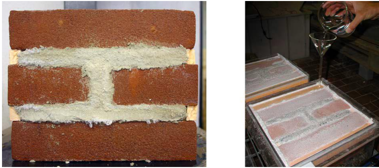
Fig. 1. Three-leaf wallette before the crystallization test (a) and stored in a plastic container at the beginning of a new crystallization cycle (b).
