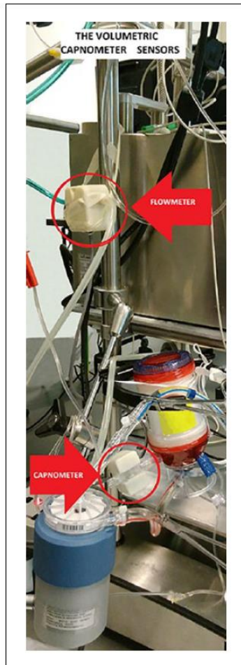
Figure 3.1. The new volumetric capnometer is applied to the ECMO machine. Top and bottom red circles are the flowmeter and capnometer, respectively.
