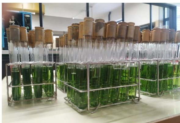
Figure 4- Racks with freshly distributed BGLB culture medium into the test tube, with the inverted Durhan tubes.
