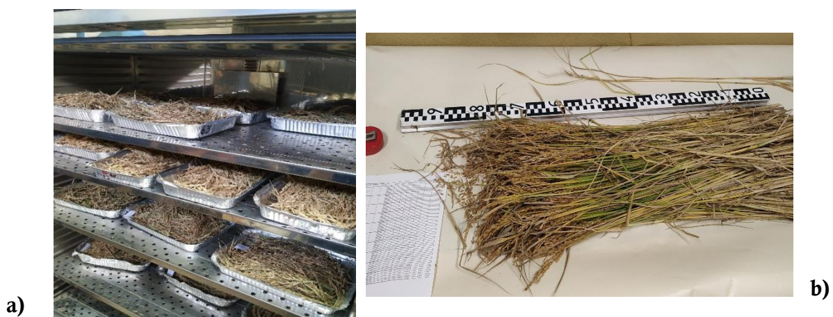
Figure 5- Photographs of the post-harvest processing. a) the samples being oven dried at 65°C; b) measuring the length of the samples with aerial part.
