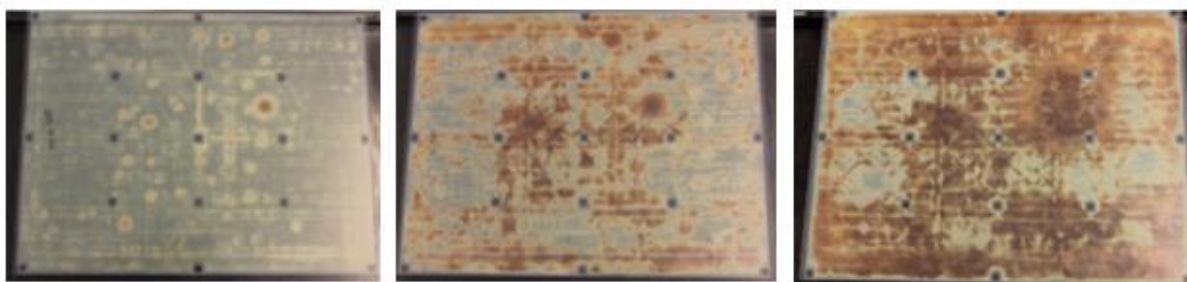
Figure 127.: Diffusers with various spacer density, left -22 pcs/mm 2 , middle - 2 pcs/mm 2 , left 0.2 pcs/mm 2 . Note rings from process pins and marks from finger touch. Small square areas inside display are intentionally made for cell gap measurement.
