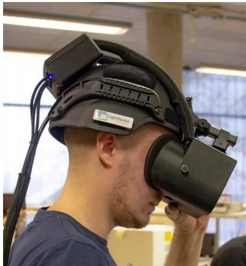
Figure 3.: A photograph of a multifocal virtual reality headset being evaluated for the first time.
