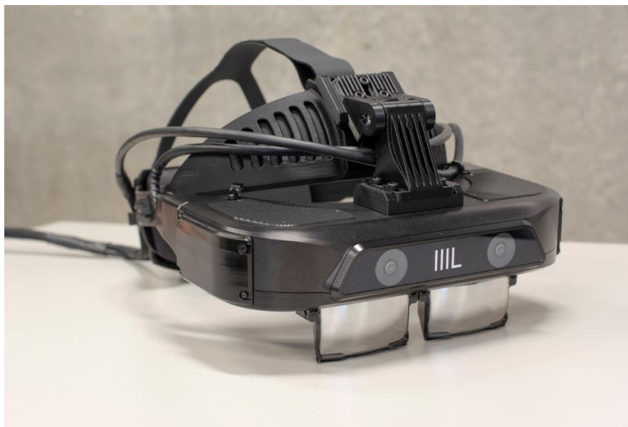
Figure 135.: Lightspace AR-HMD with multifocal liquid crystal diffusers.
