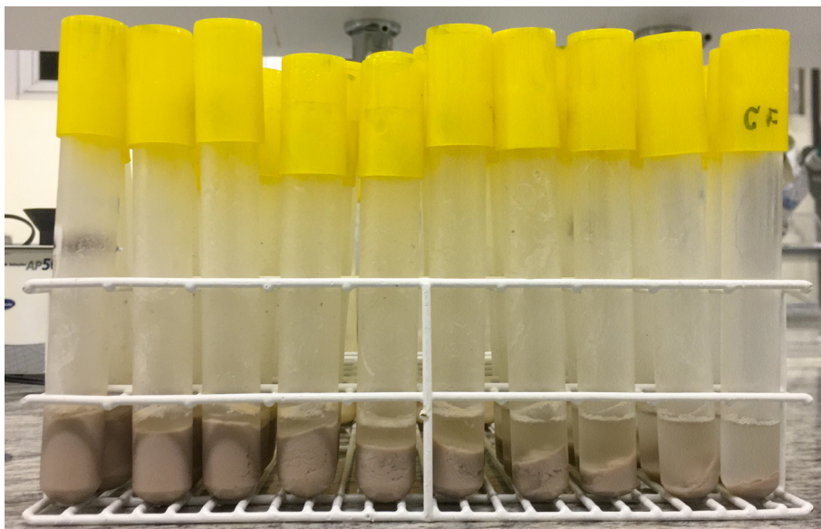
Figure 9. Gelling capacity test with tubes in decreasing order of concentration. Tubes from left to right refer to concentrations of 0.20, 0.18, 0.16, 0.14, 0.12, 0.10, 0.08, 0.06, 0.04, 0.02 g/mL.
