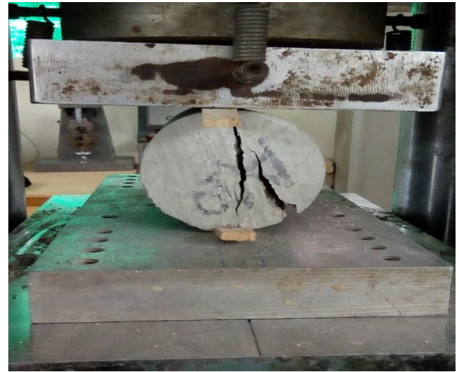
Fig. 11. Splitting tensile test
