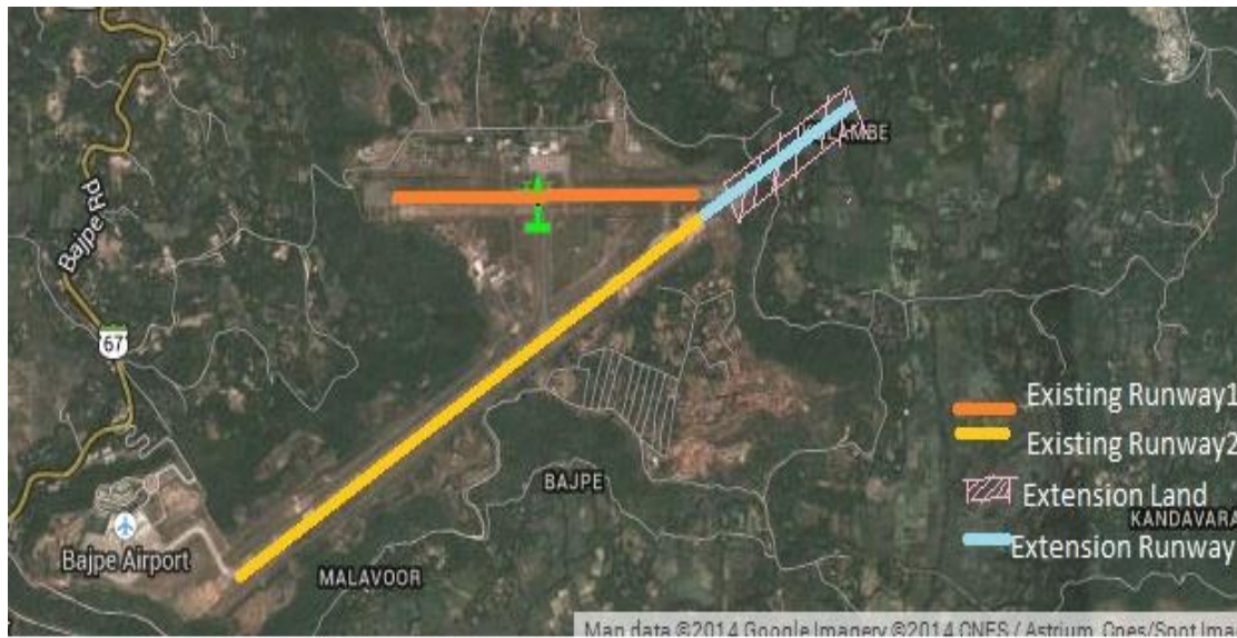
Fig .1. Map of Mangalore airport showing the existing runways and proposed extension runway.
