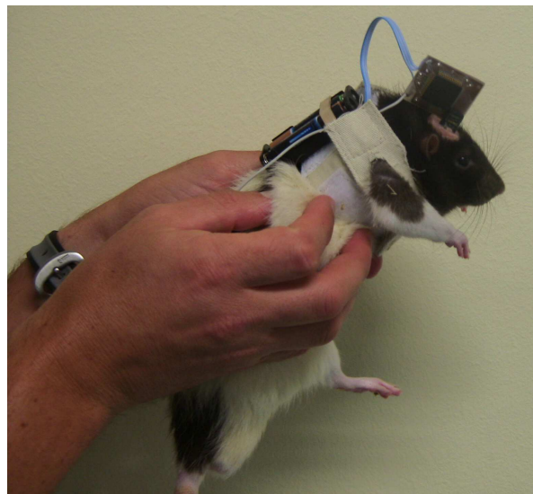
Figure 20. Arrangement for in vivo measurements. Note the headstage, the battery backpack and the whip antenna placed along the back of the animal.
