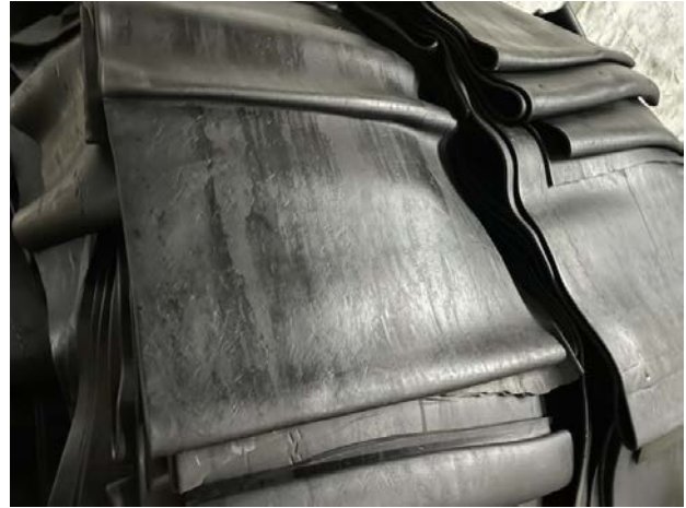
Fig. 1. Image of latex sheet used for wrapping the column
