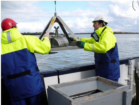
Figure 4. Day grab being deployed
