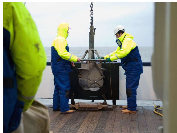
Figure 7. Box corer being deployed
