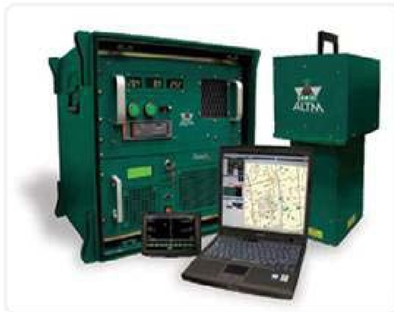
Figure 5.2. Optech Gemini Airborne Laser Terrain Mapper sensor array utilized by M.J. Harden, a Geo-eye Company (image courtesy M. J. Harden).
