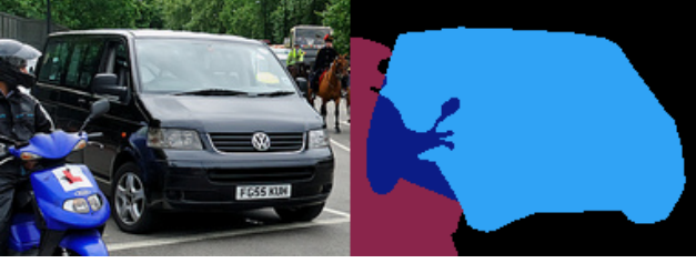
Figure 3. Illustration of the four states that a pixel can be in: Visible Foreground ( w_a = 1, z_a = 1 ) in light blue, Occluded Foreground ( w_a = 1, z_a = 0 ) in dark blue, Visible Background ( w_a = 0, z_a = 1 ) in black, and Occluded Background ( w_a = 0, z_a = 0 ) in red. Consequently, amodal segmentation of an occluded object is thus defined as Visible Foreground \cup Occluded Foreground .
