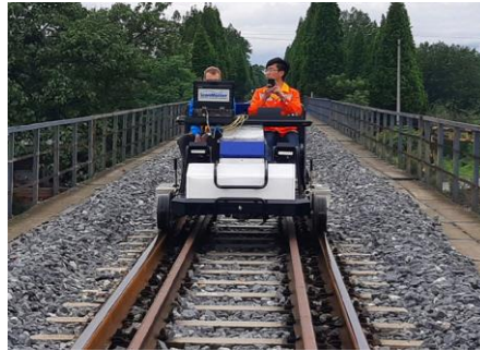
Figure 8. Automatic rail defect detection vehicle.
