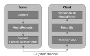
Figure 4: Client-server architecture of the MPEG-2 TS implementation.
