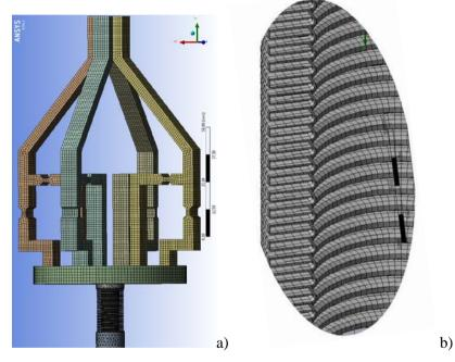
*Figure 6*: a) Mesh of the gripper with four fingers; b) Detail view regarding discretization of the FC-9 bellow.
