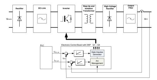
Figure 2: Schematic diagram of the DC power supply.
