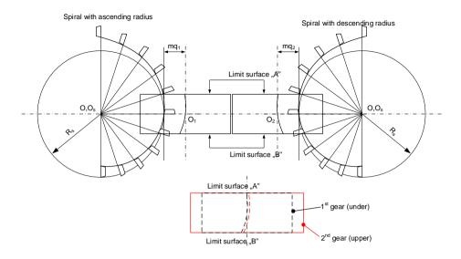
*Figure 2*: The meshing of the elements of the gear pair using a single cutter head with symmetrical positioning of the inserts.
