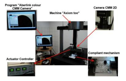
Figure 3: CMM 2D camera measurement stand.
