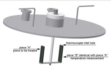
*Figure 3*: Experimental arrangement. Piece "A" is the piece to be treated; Piece "B" is an identical piece with Piece "A" located in symmetrical position with respect to the chamber axis.
