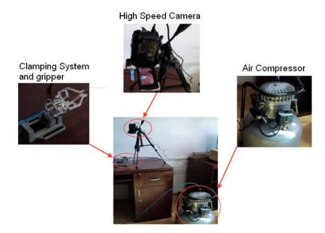
Figure 9: Experimental stand for displacement measurements.
