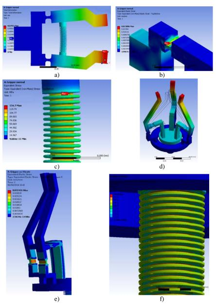
*Figure 7*: a) Total deformation of the normal gripper; b) Equivalent elastic strain of the joint; c) Equivalent stress for the FC-1 bellow; d) Normal vs. Total deformation of the gripper with three fingers; e) Equivalent elastic strain of the gripper with four fingers joints; f) Equivalent stress for the FC-9 bellow.
