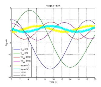
Figure 4: Stage 2: Inputs, measured outputs, estimated states.
