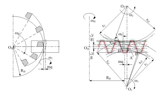
Figure 1: The sketch of the rack generating milling head and the coupling gear pair.
