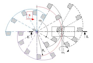
Figure 3: The cutter head and the principle of tangential feed.
