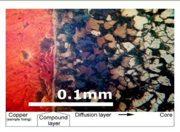
*Figure 5*: Heat treatment temperature 530°C, time-span 1 hour, magnification of the optical microscope 60x10.
