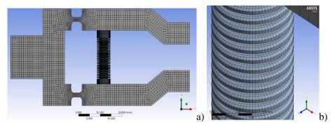
Figure 5: Discretization of the: a) normal gripper, b) FC-1 bellow.
