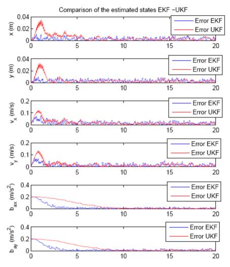
Figure 7: Comparison of UKF and EKF: estimation errors.
