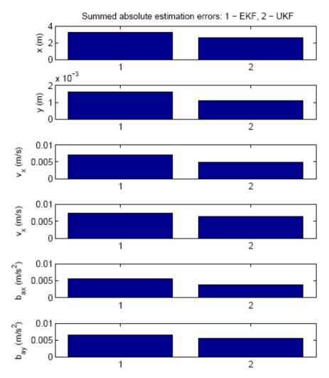
*Figure 8*: Comparison of UKF and EKF after the transients: sum of the normalized absolute values of estimation errors.
