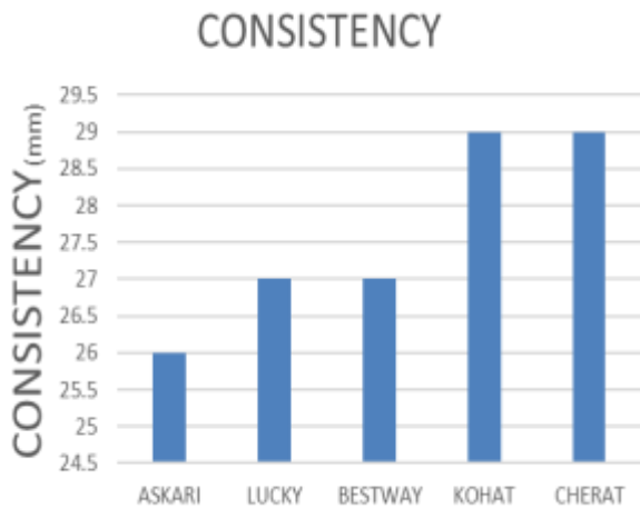
FIGURE 7. Consistency of cement
