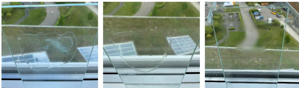
Figure S13 UV cured methoxybutenolide-1,4-butanedivinyl ether coatings using as photoinitiator 3 mol% VAPO (left), 6 mol% VAPO (middle) and 3 mol% BAPO (right). Coating formation conditions: methoxybutenolide-1,4-butanedivinyl ether (1:0.5 ratio), VAPO/BAPO (3–6 mol%), UV irradiation ( \lambda_{\text{irr}} = 395 \text{ nm} ), 20 min.
