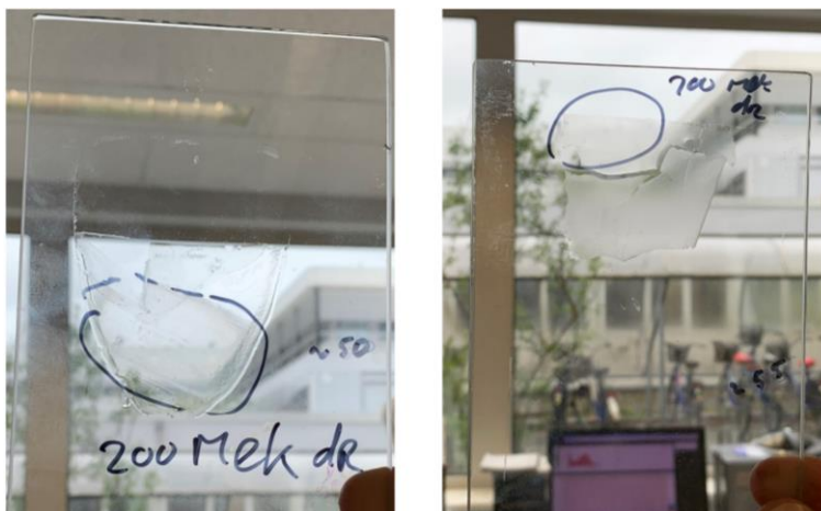
Figure S15 UV cured methoxybutenolide–1,4-butanediyl vinyl ether coatings BVEC1 (left) and BVEC2 (right) subjected to DSC, Knoop hardness measurement and MEK solvent resistance test. Only slight whitening and no other damage or deterioration of the surfaces was apparent after 200 MEK double rubs.
