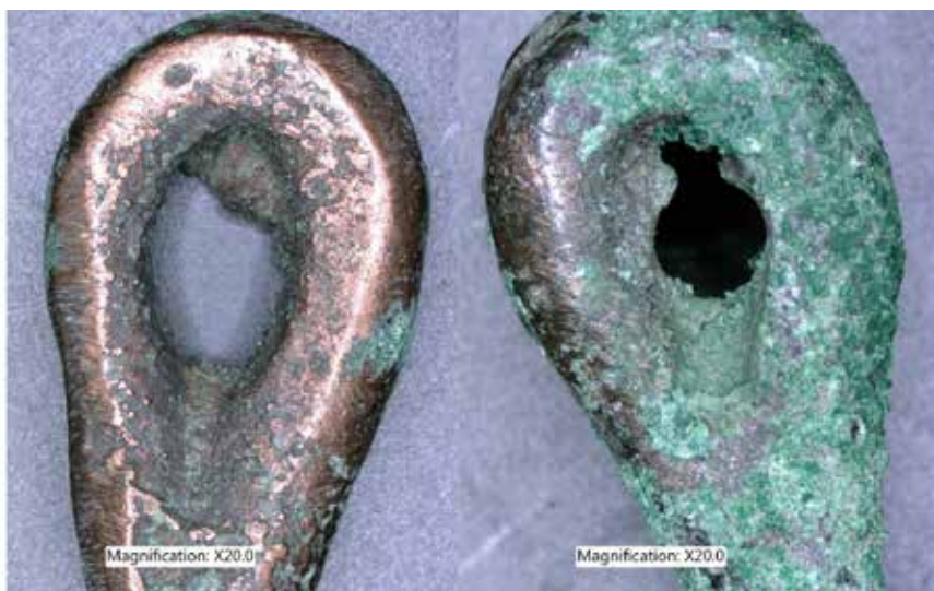
Fig. 3. The contrast of the corrosion process between two hoops of a necklace (author: Marcin Kasprowicz)
