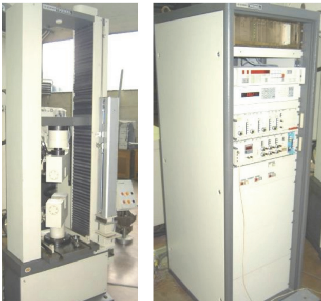
Figure 3 Electromechanical testing machine SCHENCK TREBEL RM100
