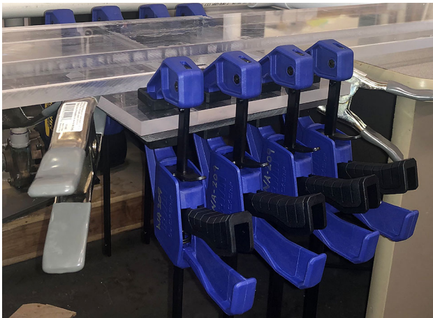
Fig. 7 Test plate clamped at the bottom of the cavity section
