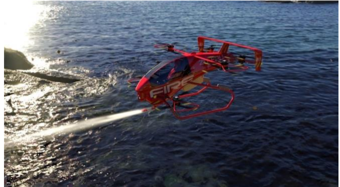
Figure 11. By combining Compressed Air Foam (CAF) and other extinguishing mediums, a small eVTOL like the one from Esprit can become an effective firefighter. Image courtesy of Esprit
