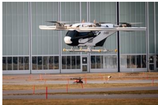
Figure 19. The CityAirbus all-electric, four-seat multicopter vehicle full-scale demonstrator conducted its first takeoff in May, 2019. Image courtesy of Airbus
