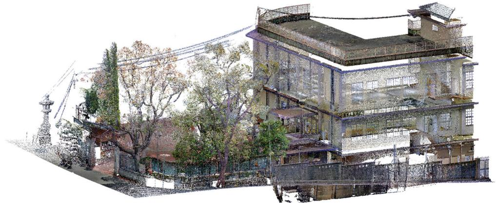
**Figure 12.** 3D laser-scanned data used in our comparative experiments of deep learning networks (10,480,242 points). The scanned target is the campus building of Kyoto Women's University, Japan.
