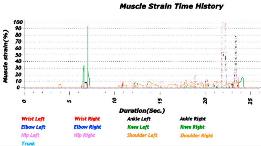
Fig. 10. Muscle Strain Time History during the execution of the short rod handling operation (including the screwing one)
