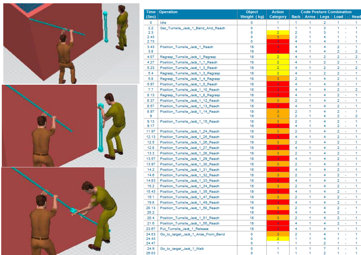
Fig. 6. Different view of the operations for fixing of the lower part of the lashing rod, for attaching the two rods and for screwing both parts together and results of the OWAS Analysis
