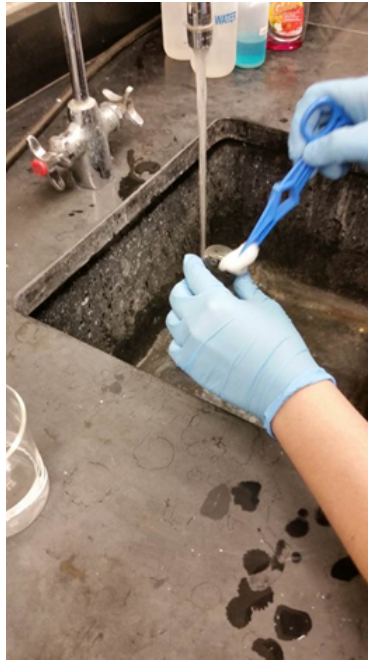
Figure 6: A typical swapping procedure for etching specimen
