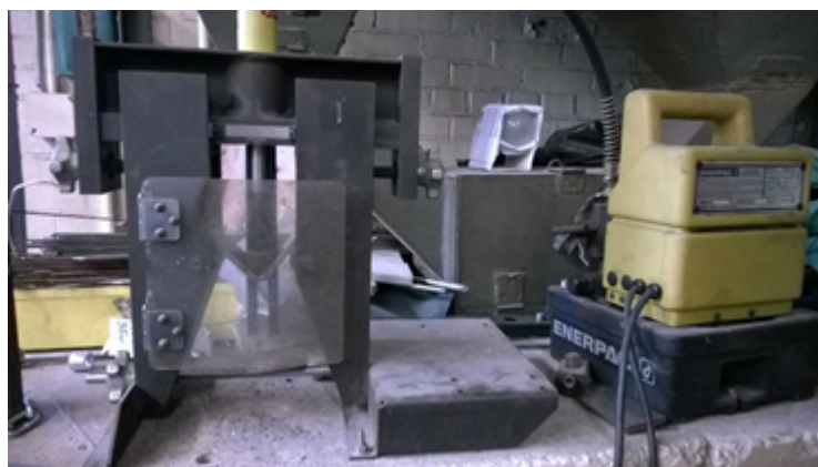
Figure 12. A guided bend test of welds.
