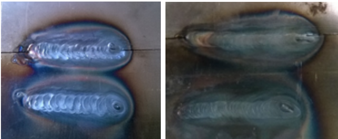
Figure 9: Two 1018 steel samples bead-on-plate and single-square groove autogenous GTAW welds. Left: weaved beads. Right: stringer beads with signs of an unsteady hand.
