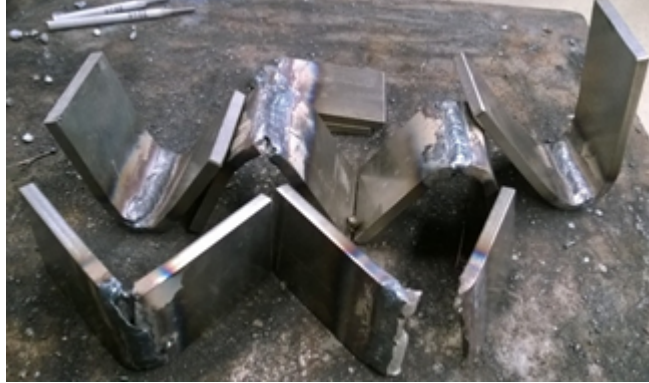
Figure 13. Some of SMAW welds after the bend test. It is easy to guess which samples were welded without grinding of the root pass to remove slag. Two samples also show effects of craters and slag inclusions created during arc termination.
