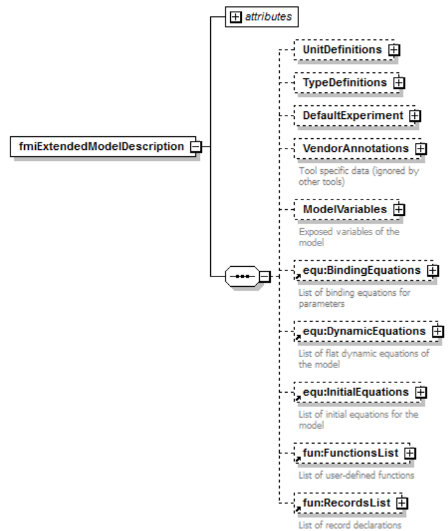
Figure 2. Overall structure of the DAE XML schema
