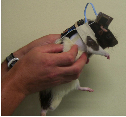
Fig. 6. Arrangement for in-vivo measurements. Note the headstage, the battery back-pack and the whip antenna placed along the back of the animal.
