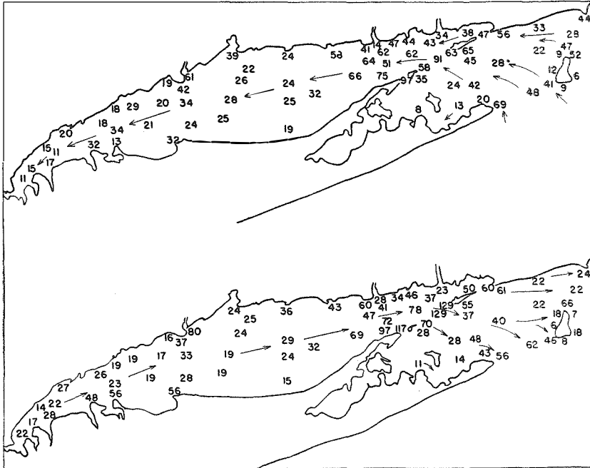
Figure 6. Average velocity in cm per second of the flood (top) and of the ebb (bottom) surface currents.
