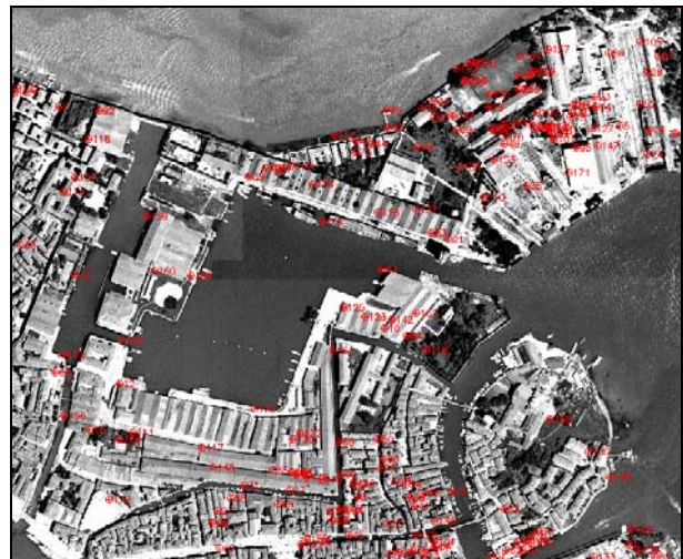
Figure 4. Nadir-looking Pléiades HR simulation generated from aerial orthophotos with superimposed the GCPs identified by the AGE algorithm
