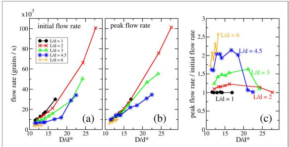
**Figure 4.** Experimental results: (a) initial flow rate, (b) peak flow rate and (c) ratio of the peak and initial flow rates as a function of the reduced orifice diameter  $D/d^*$ . The initial flow rate is measured when the material in the silo is between  $5m_{D_{\rm silo}} > m > 4m_{D_{\rm silo}}$ . The different curves correspond to particles with different aspect ratios L/d.
