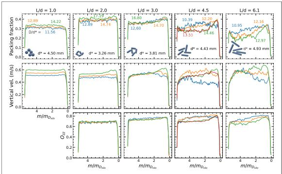
**Figure 6.** DEM results: average packing fraction (top row), vertical grain velocity (middle row) and vertical component of the orientation tensor (bottom row) as a function of the mass in the silo during the discharge process for spheres and spherocylinders with aspect ratios of L/d = 2, 3, 4.5, 6.1. The curves represent data averaged in a cylindrical region based at the orifice with a diameter of the orifice and a height of L/2.
