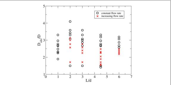
**Figure 8.** The two types of flow regimes: silo discharge with constant and increasing flow rates as a function of the particles aspect ratio L/d and the normalized silo diameter  $D_{\rm silo}/D$ .
